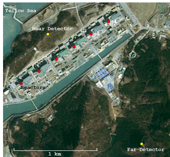
FIGURE 1. The layout of the Yonggwang experiment site. Red dots and yellow dots represent reactors and detectors, respectively.
