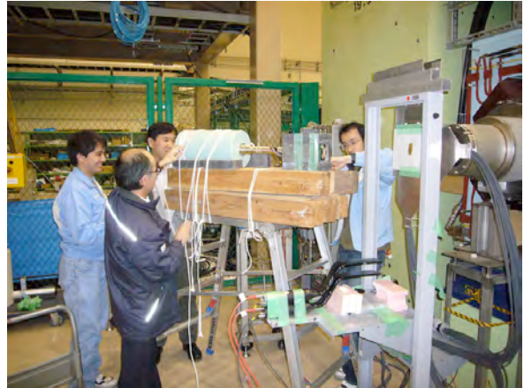
FIGURE 6. Muonic X-ray measurement system at the D2 area as a demonstration of extraction of decay negative muons. Tempo-Koban (supplied by Prof. S. Saito) was placed in front of the Ge-detector.
