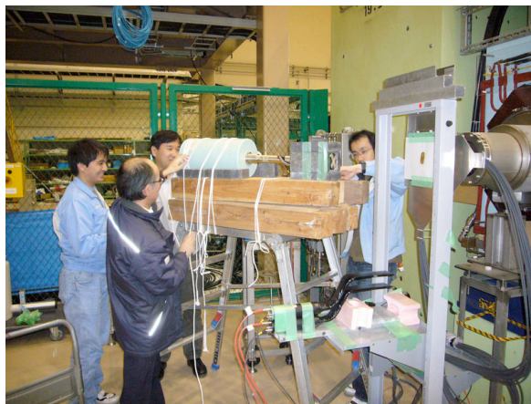
FIGURE 6. Muonic X-ray measurement system at the D2 area as a demonstration of extraction of negative decay muons. Tempo-Koban (supplied by Prof. S. Saito) was placed in front of the Ge-detector.
