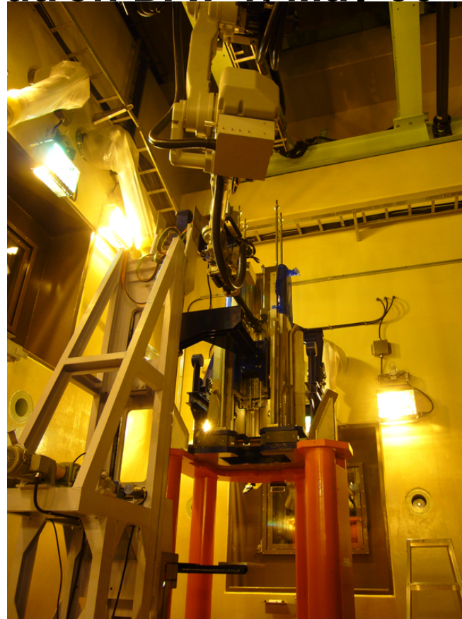
A picture of the maintenance commissioning of the target slide table in the hot cell
