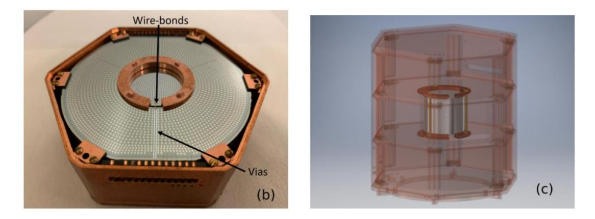
7.5 cm outer diameter, 2.8 cm inner diameter and 2.5 cm thick Ge donut having a 2.5 cm diameter and 0.1 cm thick Ge coin inside.
