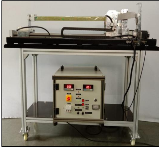
Multipoint calibration unit for hall sensors
