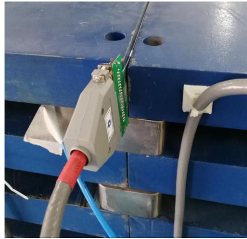
Hall probe PCB inserted for magnetic measurement
