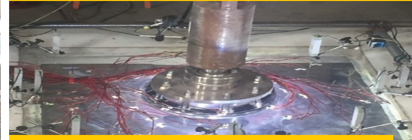
Load test of node: break at 100 tons
