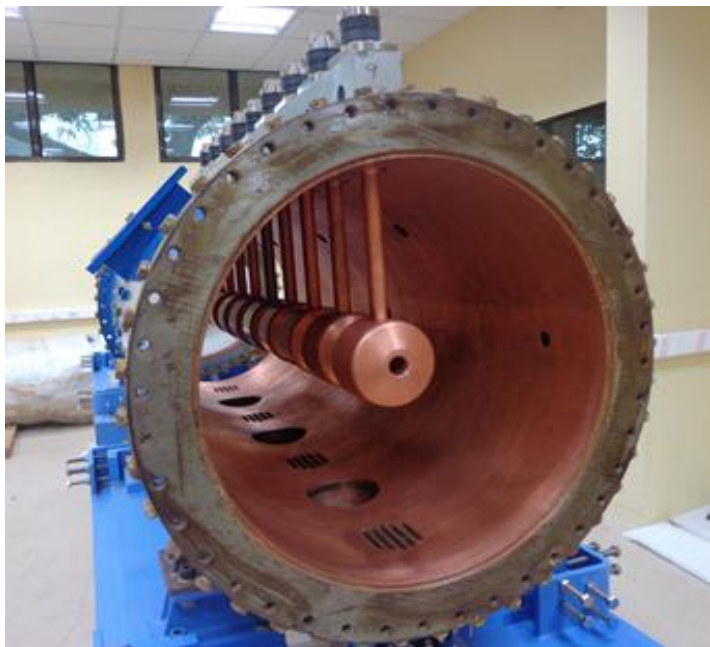
Developed Drift Tubes Linac cavity with assembled Drift Tubes
