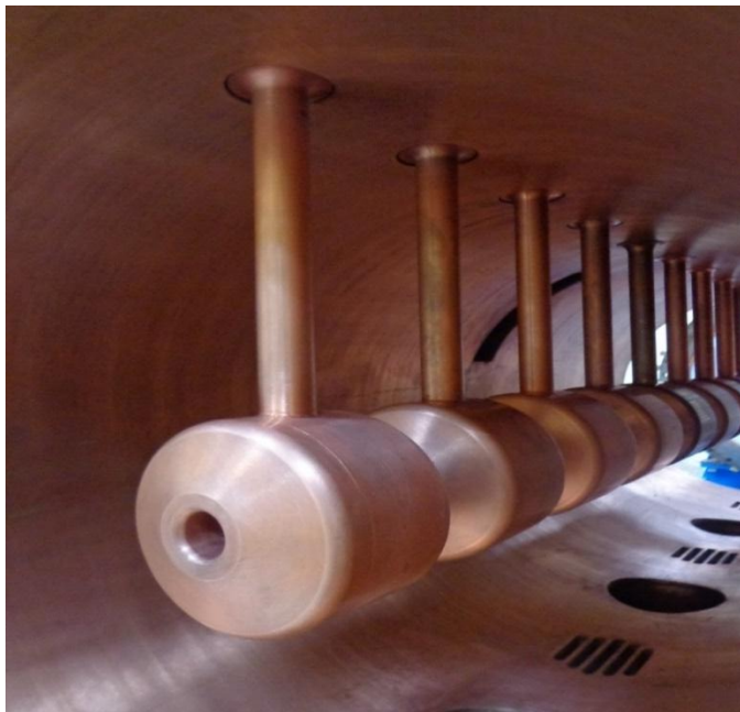
Drift Tubes aligned concentrically along the DTL cavity axis
