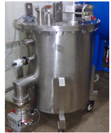
130 mm warm bore cryogen free SC magnet for High Frequency RF device
