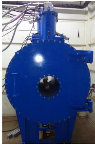
300mm cryogen free SC magnet for MHD experiments
