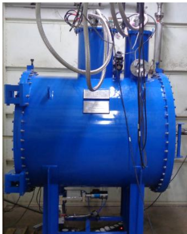
300mm cryogen free SC magnet for MHD experiments
