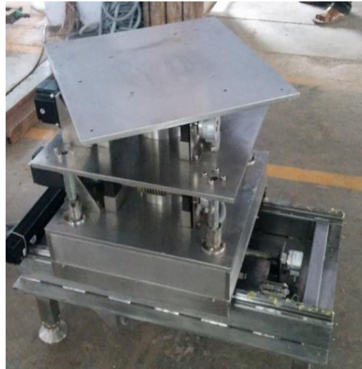
X-Z-θ motion stages which can carry 500 Kg max load
