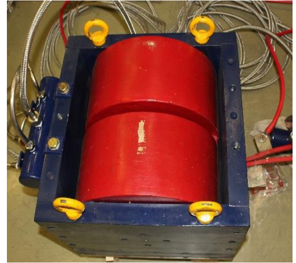
Electromagnet with hydraulic and Electrical connections
