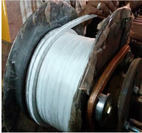
Jig for winding 12mm × 12mm hollow conductor XMCD Dipole Electromagnet
